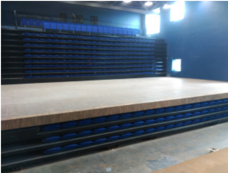
FOLDABLE FOOT, UPHOLSTERED SEATING. AUTOMATIC LIFTING AND FOLDING OF FOOT
